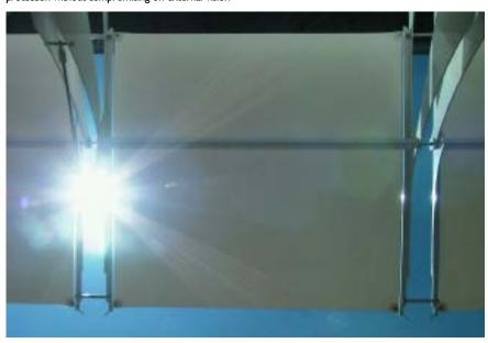
Test rig for Zurich Airport, Switzerland utilising various fabric and perforated metal fins
